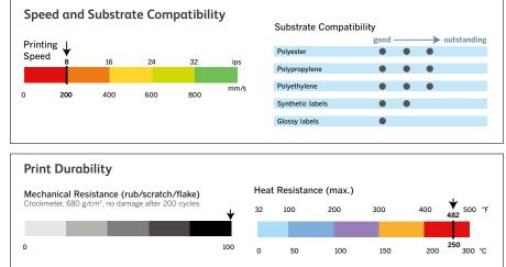
Videojet evaluation of observed performances of the Chemical-resistant Ribbon with optimized printer setting and receptors.
